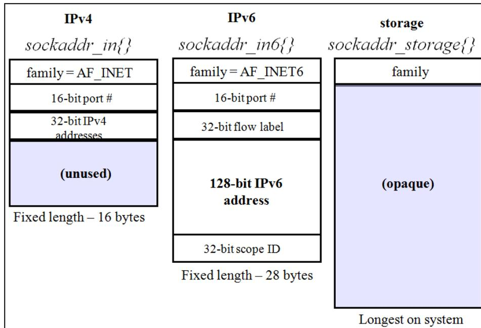
**Figure 4: Protocol Specific compared to Protocol Independent - Storage**
