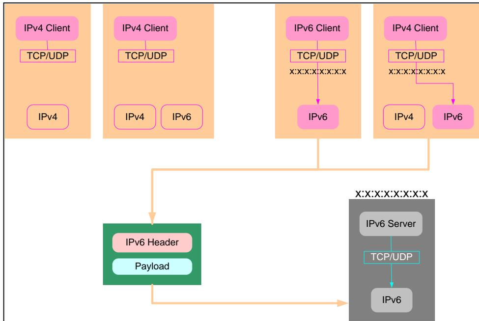
**Figure 6: Mixed Clients and IPv6 Server in an IPv6 Only Node**
