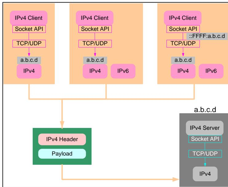
**Figure 5: IPv4 Clients and IPv4 Server in an IPv4 Only Node**
