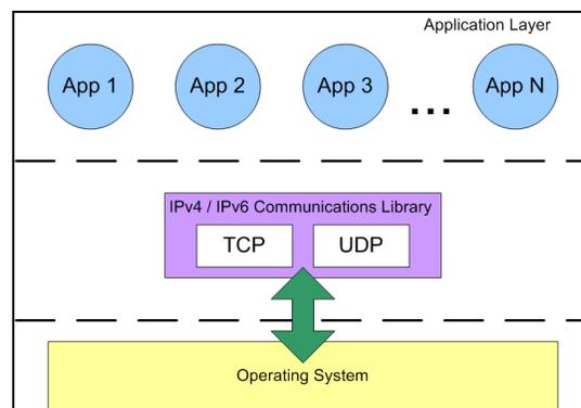
**Figure 3: Using a Communications Library to Separate Applications from the IP Address Structure**
